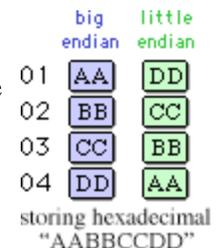
**Big endian** stores scalars in their “natural order”, with most significant byte in the lowest numeric byte address. Examples of big endian processors are the IBM System 360 and 370, Motorola 680x0, Motorola 68300, and most RISC processors.
